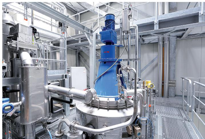
Fig. 2: The strength of short path distillation is that it is gentle on unsaturated fatty acids and yet provides effective purification. (Photo®: Nutriswiss)
